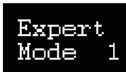
The E-PIPE one can be used in 5 different modes. However, to keep the menu as short and simple as possible, 3 of the 5 modes are only available when Expert mode is set to 1. The name Expert mode means that the use of the additional operating modes requires additional knowledge about their functionality.
